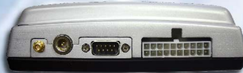
GPS GPRS DISPLAY POWER and I/O
